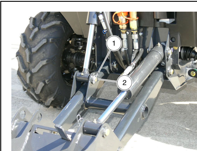
Figure 19-7 Remove Attachment Cylinder Retaining Pin
