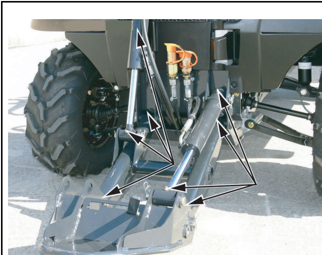
Figure 10-4 Lubricate Grease Zerks located on Cylinder and Attachment Arm Ends
